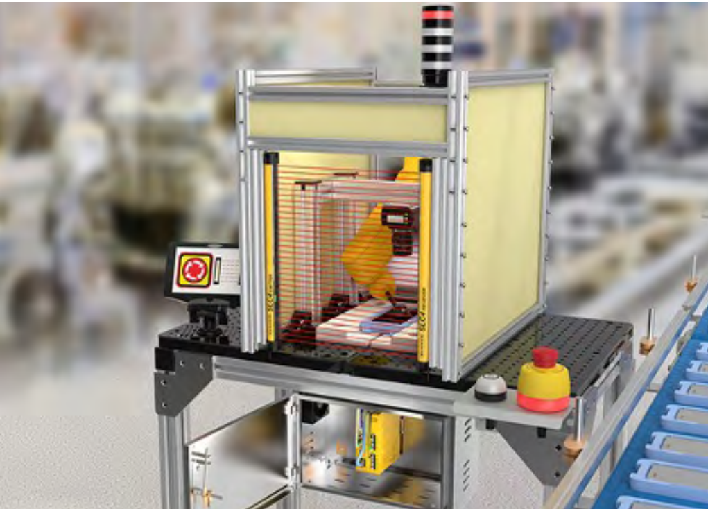
Figure 1: Shown here is a Banner Engineering SC10 Series safety controller designed to deliver the functionality of three safety relay modules. (Image source: Banner Engineering)
