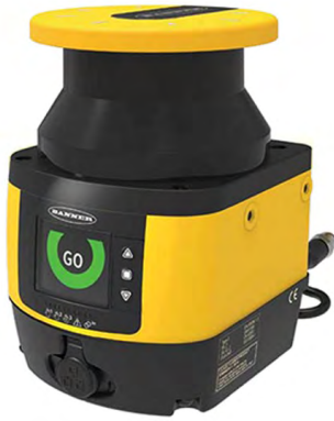
Figure 2: The Banner Engineering SX5-B safety laser scanner has a maximum range for safety and warning zones of 5.5 m and 40 m, respectively. It can provide 275 degrees of coverage and is immune to ambient light and dust. (Image source: Banner Engineering)
