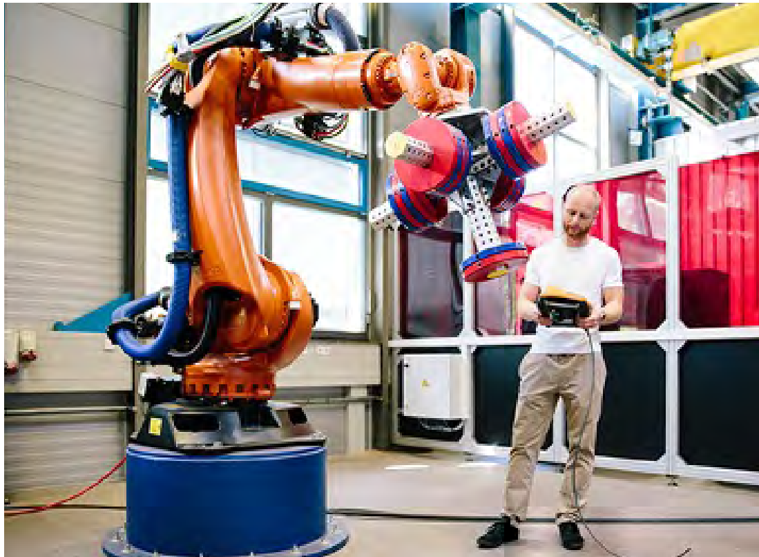
Figure 2: Particularly unique are safety circuits associated with robotics – especially for robotics that employ teach pendants (as shown here) as well as collaborative robots.
