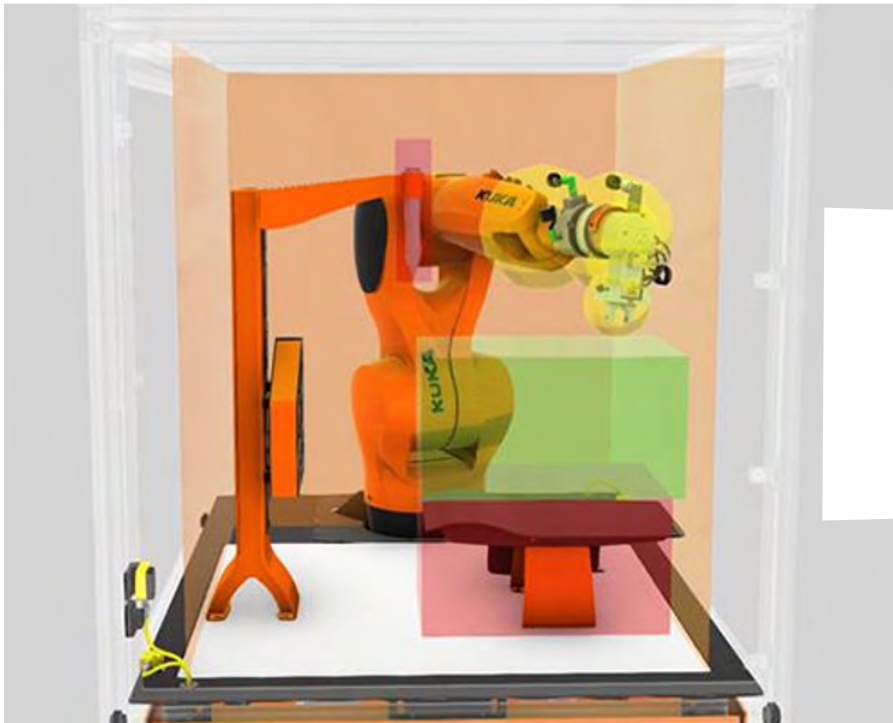
Figure 8: Developers can refine position related safety monitoring using KUKA. SafeOperation software with which they can define an operating area and model end-effector tools. (Image source: KUKA Robotics)
