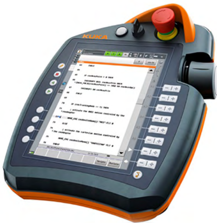
Figure 7: The KUKA robot kits include a smartPAD touch operator panel to enable hand-guided control where appropriate. (Image source: KUKA Robotics)
