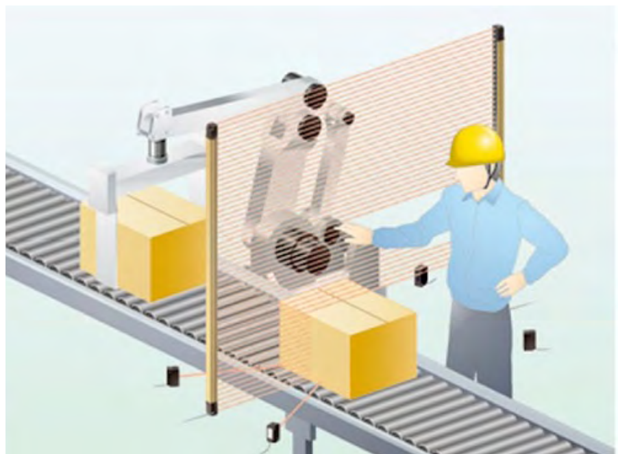
Figure 1: Proximity sensors help discriminate between a passing workpiece and intrusion by a human operator.
