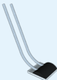
Invert welded & bent wires (U)
