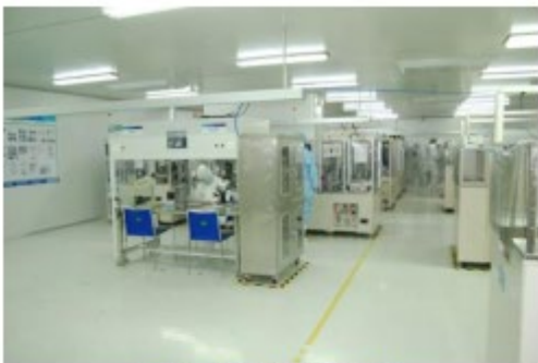
Clean room Level <10,000
