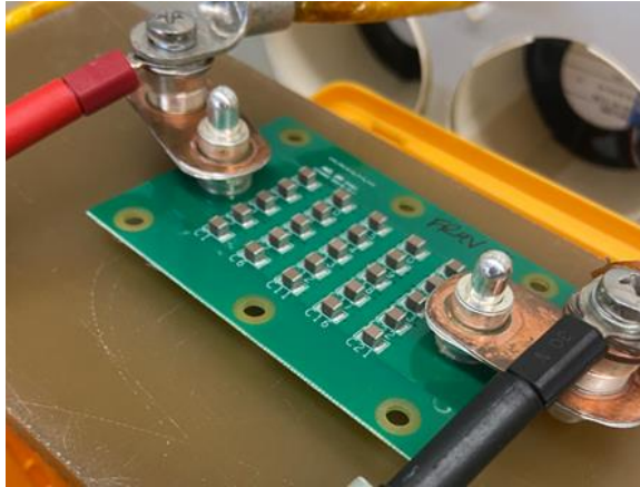
Figure 15 – 5x5 Array with no heat sink (NS)
