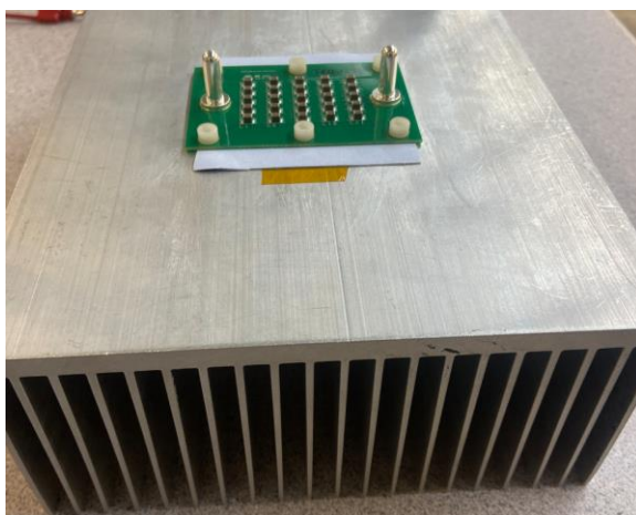
Figure 17 – 5x5 Array with large heat sink (HS1)
