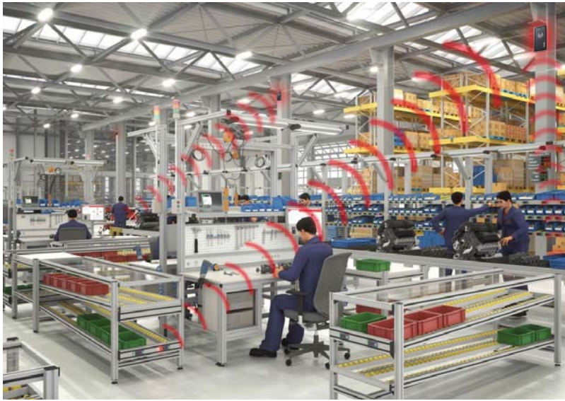
Figure 2. One of the first user examples of an integrated wireless solution was an E-Kanban system for the automatic replenishing of work stations
