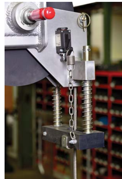
Figure 2. A wireless pull wire switch causes the winch to stop when the hook block reaches its upper limit
