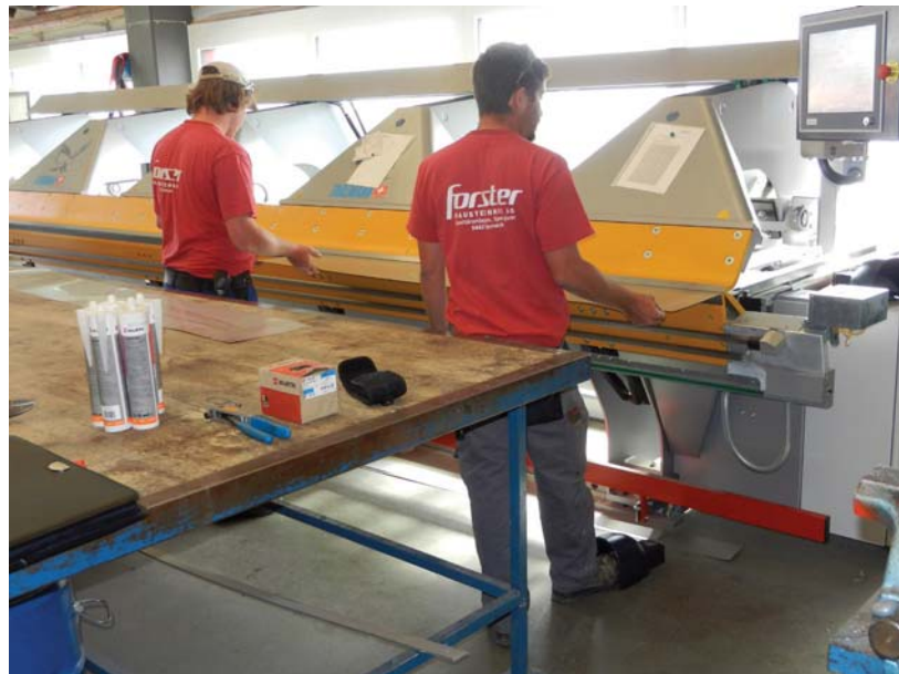
Figure 1. Forster Haustechnik AG uses a modern swing-folding machine to create façades.
