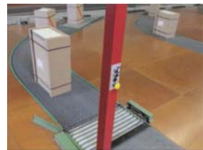
Figure 3. Via a wireless switch, the user sends the information that a consignment has been loaded from an accumulating conveyor
