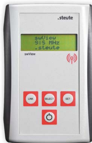
Hand-held Field Strength Monitor aids in system installation and maintenance
