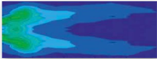
Air Distribution without Air Guiding System illustration
