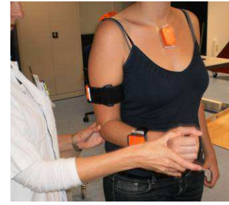
Fig. 10. Wireless measurement of scapular dyskinesis with the MTw.
