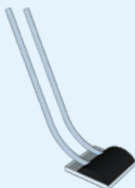
Invert welded & bent wires (U)
