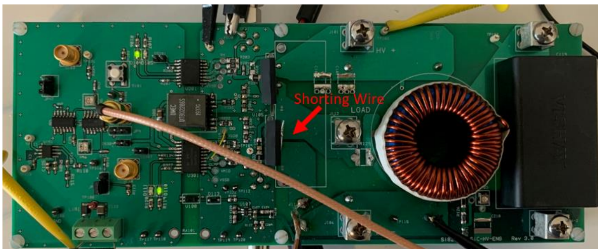
FIGURE 1: TEST SETUP WITH LOWER SiC MOSFET SHORTED (UPPER SiC MOSFET IS DUT)
